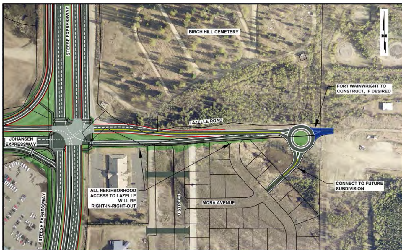
Figure 6: Design Options for Lazelle Road and City Lights Boulevard with Echelon Alternative
