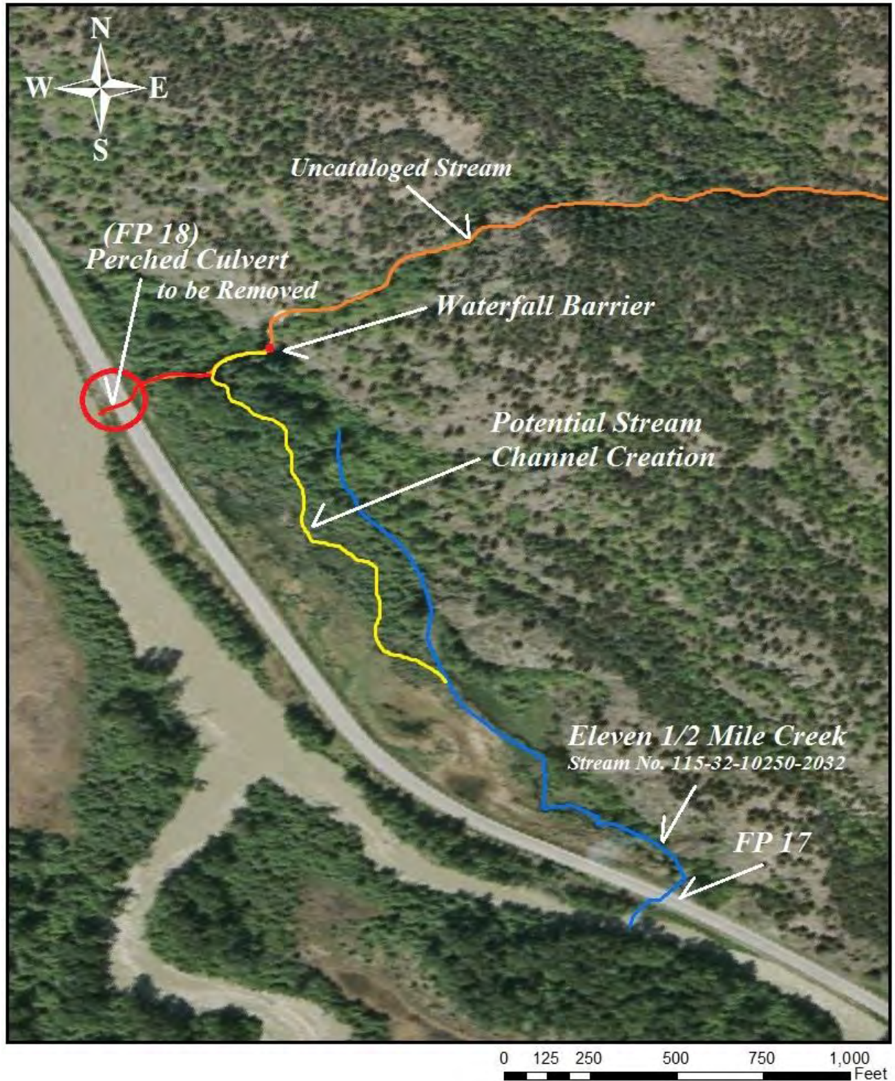
Figure 4. Aerial diagram of proposed mitigation channel.
